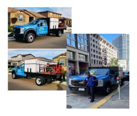
This F550 Pressure Washing Truck is called "The Beast". This one-of-a-kind truck holds a 1000 Gallon Tank! Double-Rigged with two 200ft hoses that can cover 400ft worth of sidewalk in half the time! Perfect equipment to handle the demand of our bricked sidewalks of Market Street.
